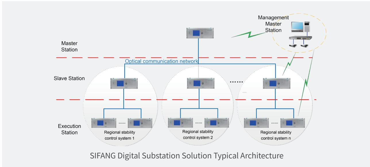
Designed with a three-tier architecture, the system leverages fiber-optic interconnections for multi-station coordination. The primary functional units are the Stability Control IEDs, which provide comprehensive system monitoring and command execution. These IEDs are versatile, functioning as Master, Slave, or Execution stations based on the network topology.
