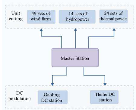
1 master station and 89 remote execution stations implementing DC modulation and selective generation tripping. Provides a high-reliability defense against severe AC/DC faults and effectively prevents cascading failures.
