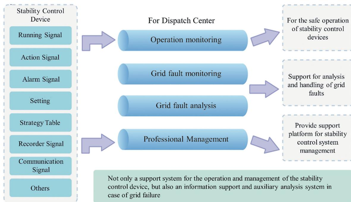
The SIFANG Stability Control Management System can integrate stability control devices from different manufacturers and models through two access modes, enabling centralized monitoring and management at the dispatching center:
